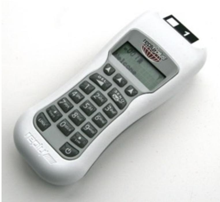
The Reply Mini+ keypad is a wearable keypad designed to be affixed to the delegate lanyard. The device is simple to use and its relative size makes it easy to transport and deploy. Vote confirmation is given by a coloured led.
